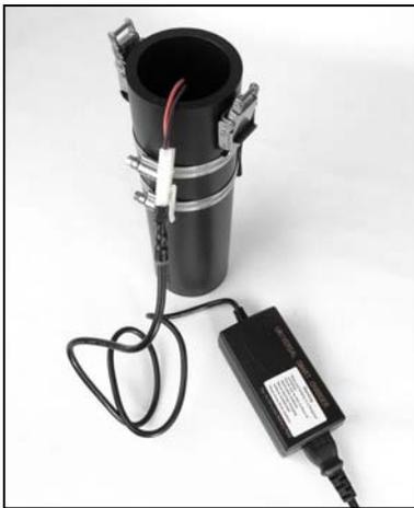
2. Connect battery canister to universal charger by tamiya connector. There is no chance to make any mistake because of the connector shape.
